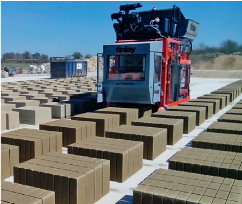
The new 'egg-laying' block plant is delivering a substantial increase in production at our recently acquired Huntsmans quarry at Naunton in Gloucestershire.
